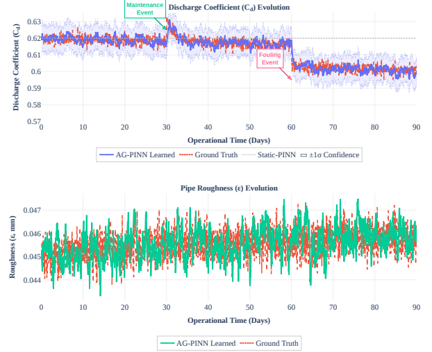
Figure 1. Evolution of physical parameters over 90-day system aging. (Top) Discharge coefficient ( \hat{C}_d ): AG-PINN (blue) adaptively tracks true degradation (red dashed) from 0.62 to approximately 0.60, while Static-PINN (gray) remains fixed. (Bottom) Pipe roughness ( \hat{\epsilon} ): AG-PINN (green) follows the fouling accumulation trend. The adaptive mechanism maintains sub-0.5% FPR throughout.
